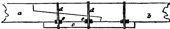
Fig. 88—Represents a scarf joint for a cross strain secured at bottom by a piece of timber c confined to the beams by iron hoops d, d and keys e, e .
